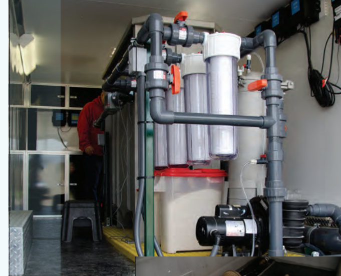
These pictures show the internal components of a DE vacuum filtration system.
